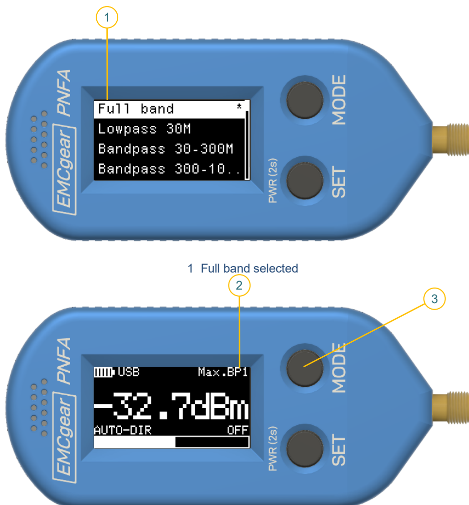
2 Strongest band 3 MODE: short press to cycle wideband filters
